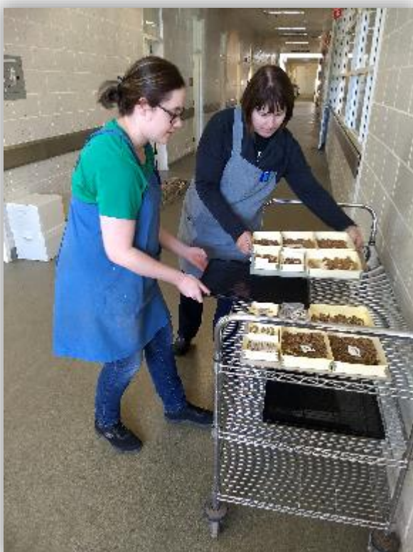
FIGURE 47: CONSERVATORS HEATHER RARDIN AND FRANCIS LUKEZIC SLIDE A CR CASSETTE UNDER A PREPARED TRAY PRIOR TO X-RADIOGRAPHY.
