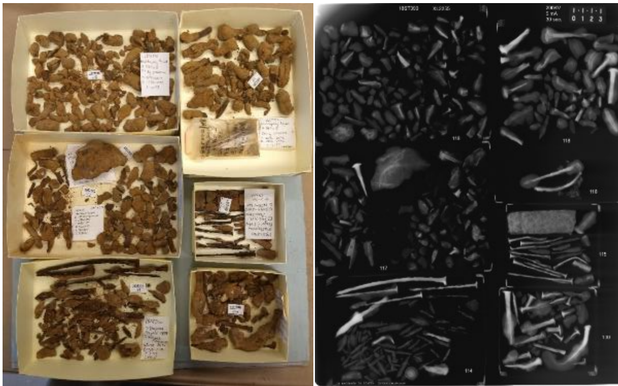
FIGURE 40: IF SMALLER BOXES OR TRAYS ARE AVAILABLE, IT DOESN'T TAKE MUCH TIME TO REMOVE ARTIFACTS FROM BAGS AND SPREAD THEM OUT TO PREVENT OVERLAP. VISIBILITY IS GOOD ON THE RESULTING X-RAY, THOUGH THE X-RAY IS A BIT MORE DIFFICULT TO CATALOG AND LABEL WHEN ARTIFACTS ARE NOT MORE CAREFULLY LINED UP.
