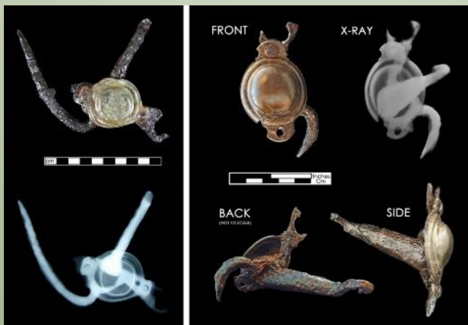
FIGURE 1: THESE TWO CURB BITS ILLUSTRATE HOW X-RAYS DIFFER WHEN ARTIFACTS LIE FLAT (LEFT) COMPARED TO THOSE THAT DO NOT (RIGHT). THE LATTER HAS A MOUTHPIECE THAT POINTS UP WHEN THE BIT IS PLACED WITH THE BOSS SOMEWHAT FLAT ON THE FILM. WHILE THE CHEEK PIECE IS SHOWN WITH DECENT ACCURACY, THE VISUAL REPRESENTATION OF THE MOUTHPIECE IN THE X-RAY IS DISTORTED BY THE PERSPECTIVE.
