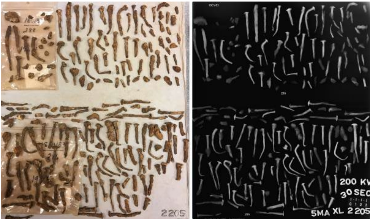
FIGURE 40: LAYING OUT ARTIFACTS FOR X-RADIOGRAPHY TAKES TIME, BUT THE RESULTING X-RAY IMAGES ARE THE EASIEST TO CATALOG, ESPECIALLY IF YOU LEAVE ROOM BETWEEN NAILS TO ADD LABELS.
