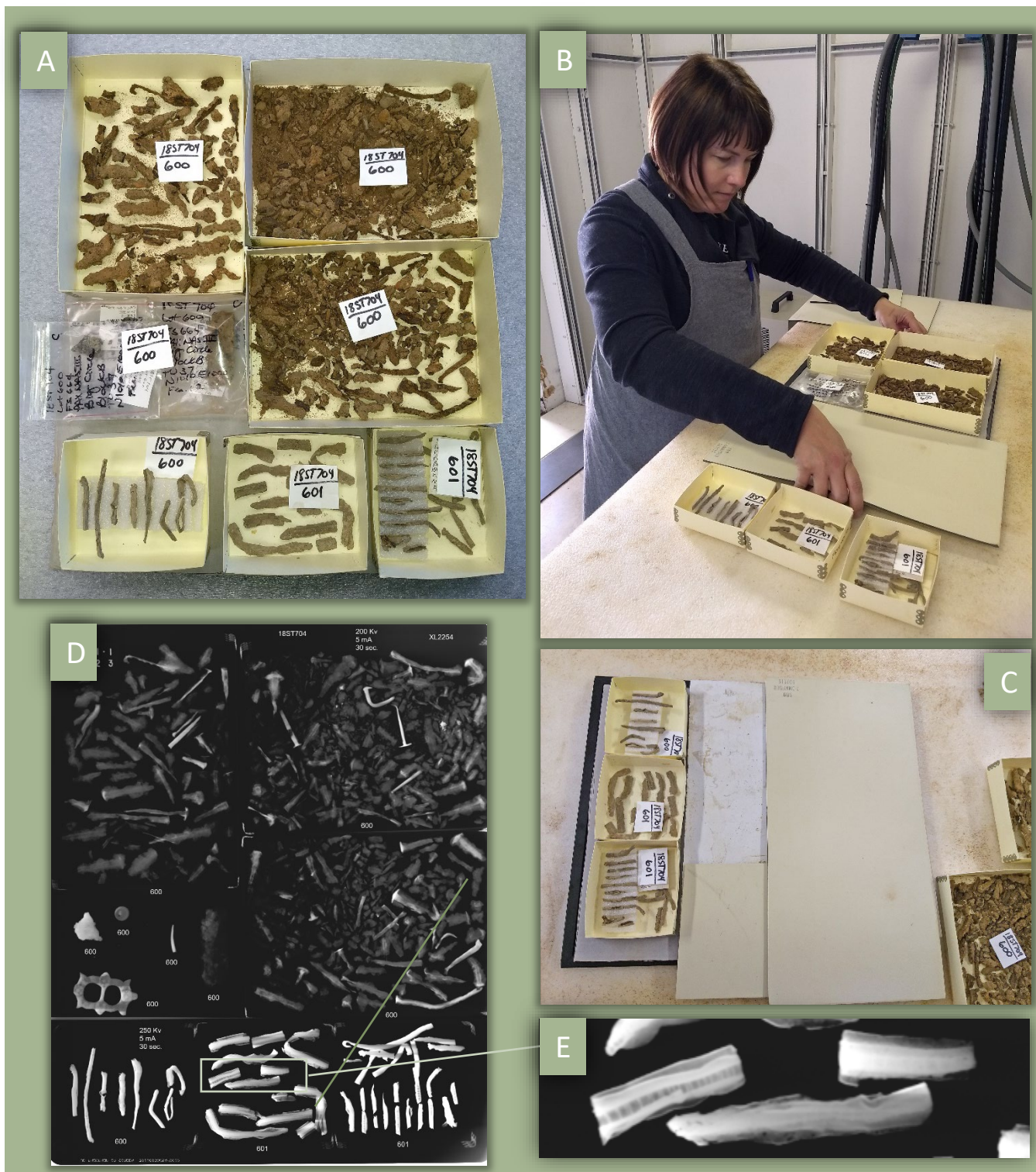
FIGURE 17: FOR THIS X-RAY LAYOUT, IRON AND COPPER ALLOY ARTIFACTS ARE GROUPED ON THE TOP TWO THIRDS OF THE PLATE WHILE WINDOW LEADS ARE LINED UP AT THE BOTTOM (A). CONSERVATOR FRANCIS LUKEZIC USED DIFFERENT SETTINGS FOR THE DIFFERENT MATERIALS. FIRST, SHE REMOVED THE WINDOW LEADS AND BLOCKED OFF THE PLATE WHERE THEY WOULD SIT, X-RAYING ONLY THE IRON AND COPPER AT 200KV (B). THEN SHE SWITCHED THE AREAS TO BE EXPOSED AND X-RAYED ONLY THE WINDOW LEADS AT 250KV (C). IN THE RESULTING X-RAY (D), IT IS POSSIBLE TO SEE WHETHER MARKS ARE PRESENT ON SOME OF THE WINDOW LEADS (E).
