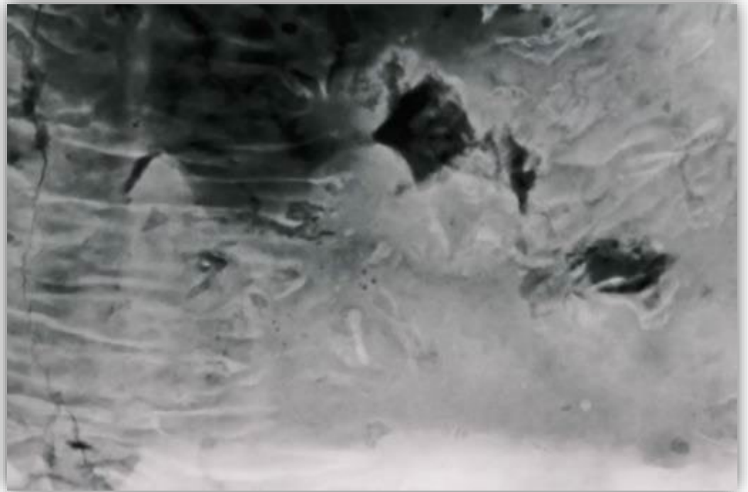
FIGURE 26: THIS IMAGE ILLUSTRATES ANOTHER TYPE OF CASTING FAILURE CAUSED BY THE METAL BEING TOO COOL. FLOW LINES ARE VISIBLE WHERE THE METAL SOLIDIFIED UNEVENLY.
