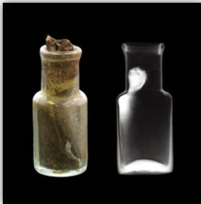
FIGURE 16: THIS VIAL WAS FOUND WITH A WAD OF TEXTILES, BUTTONS, AND PERSONAL ITEMS THAT BELONGED TO A CIVIL WAR SOLDIER. WHEN THE WAD WAS X-RAYED, THE VIAL'S CONTENTS SHOWED AS A BRIGHT SPOT, SUGGESTING THAT IT WAS ONE OF THE 19TH-CENTURY'S POPULAR MERCURY-BASED REMEDIES.
