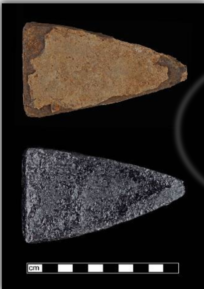
FIGURE 27: THIS INSERT FOR A BOX IRON LOOKS SOLID TO THE EYE (SHOWN BEFORE AND AFTER TREATMENT AT LEFT), BUT X-RAYS REVEALED HOLLOWES RESULTING FROM THE CASTING PROCESS. INSTEAD OF FILLING THE MOLD COMPLETELY, SOME TRAPPED AIR REMAINED WHEN THE CAST METAL COOLED.
