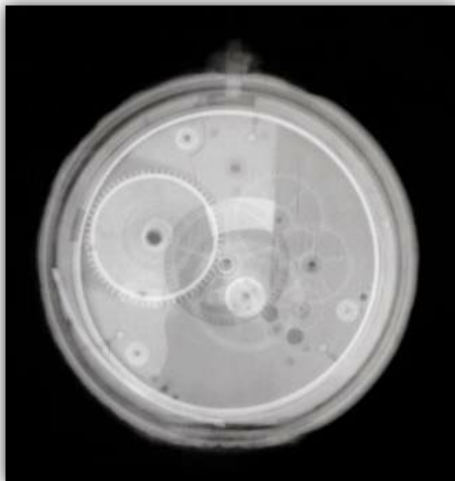
FIGURE 19: THE MANY DELICATE GEARS WITHIN A POCKET WATCH ARE READILY VISIBLE IN AN X-RAY.
