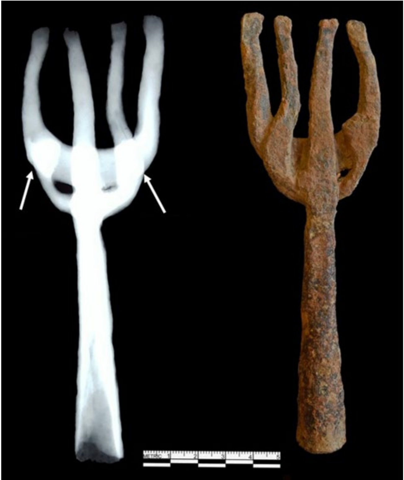
FIGURE 23: FROG GIG. ARROWS POINT TO AREAS THAT ARE HEAT-JOINED. PHOTO BY KERRY S. GONZÁLEZ, COURTESY NORTH CAROLINA DEPARTMENT OF TRANSPORTATION
