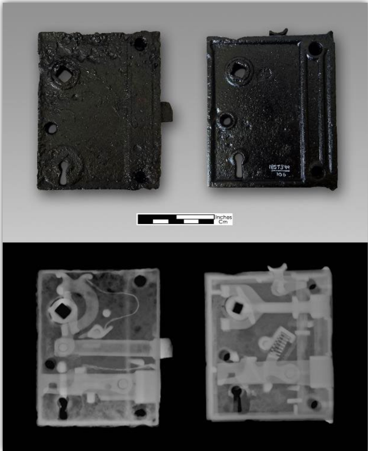
FIGURE 20: THESE TWO DOOR LOCKS LOOK QUITE SIMILAR ON THE OUTSIDE, BUT X-RAYS REVEAL DIFFERENCES BETWEEN THE MECHANISMS INSIDE.
