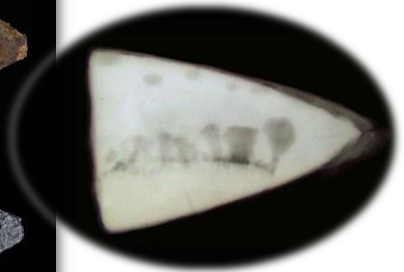
FIGURE 27: THIS INSERT FOR A BOX IRON LOOKS SOLID TO THE EYE (SHOWN BEFORE AND AFTER TREATMENT AT LEFT), BUT X-RAYS REVEALED HOLLOWES RESULTING FROM THE CASTING PROCESS. INSTEAD OF FILLING THE MOLD COMPLETELY, SOME TRAPPED AIR REMAINED WHEN THE CAST METAL COOLED.
