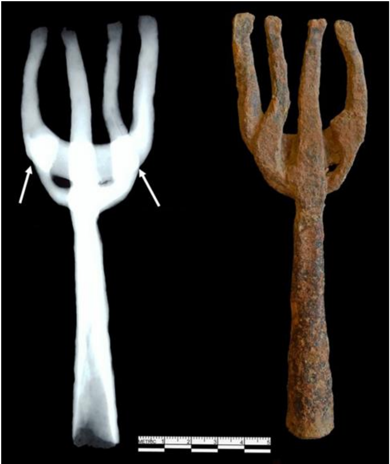
FIGURE 23: FROG GIG. ARROWS POINT TO AREAS THAT ARE HEAT-JOINED.
