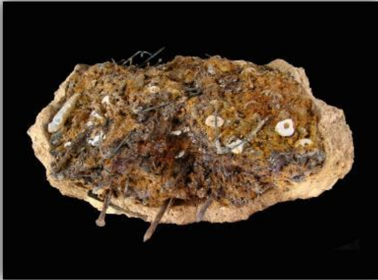
FIGURE 35: SEVERAL SEWER PIPES FROM AN AREA OF BALTIMORE THAT WAS THE HOME TO A LAUNDERING BUSINESS IN THE EARLY 20 TH CENTURY WERE CLOGGED WITH CORRODED NAILS, PINS, BUTTONS, BOLTS, AND OTHER DEBRIS. X-RAYS OFFER A LOOK INSIDE THE CONCRETION WITHOUT DISMANTLING IT. UNFORTUNATELY THE LOW-DENSITY ARTIFACTS TRAPPED IN THE CORROSION ARE NOT VISIBLE ON THE X-RAY. FOR EXAMPLE, SHELL BUTTONS ARE VISIBLE ON THE SURFACE OF THE CONCRETION, BUT NONE ARE VISIBLE ON THE X-RAY. NO DOUBT THERE ARE OTHER ORGANICS THAT EXIST WITHIN THE CONCRETION EVEN THOUGH THEY ARE UNINTENTIONALLY “ERASED” IN THE X-RAY IMAGE.
