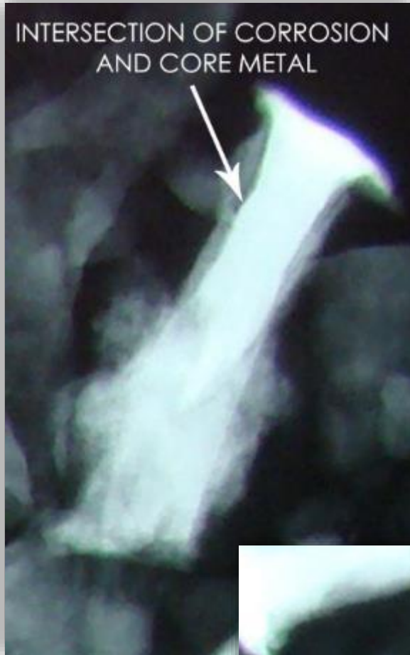
FIGURE 29: THIS NAIL IS ALMOST COMPLETELY MINERALIZED, BUT THE ORIGINAL SURFACE IS STILL DISCERNABLE AS A BRIGHT LINE THAT MAKES ACCURATE MEASUREMENTS POSSIBLE.
