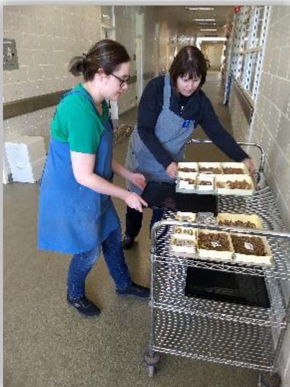
FIGURE 48: CONSERVATORS HEATHER RARDIN AND FRANCIS LUKEZIC SLIDE A CR CASSETTE UNDER A PREPARED TRAY PRIOR TO X-RADIOGRAPHY.
